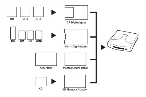
Note: The Pocket UDD is not compatible with Wireless Broadband card, Panasonic P2 card, SRAM card and Linear Memory card.
